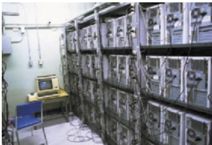
Figure 6. Cobalt, a Beowulf-class supercomputer built from 94 commodity workstations.
